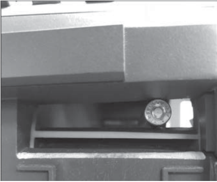
Hopper Jam (side panel removed)
