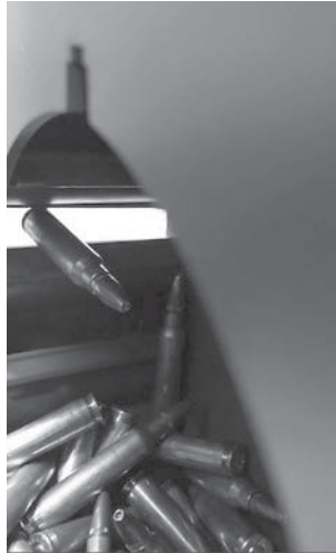
Hopper Jam (view from hopper door area)
