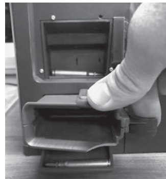
Ammo Release Lever dispenses 3-4 cartridges into tray
