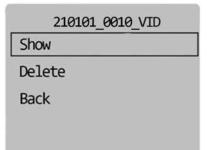
If you select the Show option in a video, you can press the Enter button to pause or continue the video. To exit video playback, press and hold the Enter button for 3 seconds.
