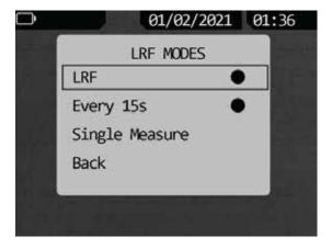
The LRF has two sampling modes: every 15s to take samples every 15 seconds, and single mode to take only one sample. Go to the desired option and click the Enter button to select.
