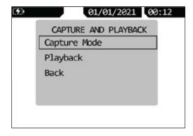
Go to Capture Mode option and select the capture mode you want, as shown in the image. Press the Enter button to select.
