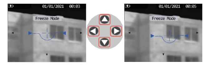
After freezing the image, you can move the reticle across the image with the arrow buttons.
