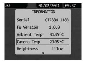
You can change the temperature unit from °F to °C. To change the temperature unit, press the Enter button to go to Main Menu, select System Settings and find the Temperature Unit option. To change the temperature go to Temperature Unit and press the arrow button.
