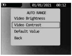
When you enter the Video Brightness or Video Contrast options, the following images will be displayed on the screen. To change the parameters, press the cursor buttons until you get the desired image.
