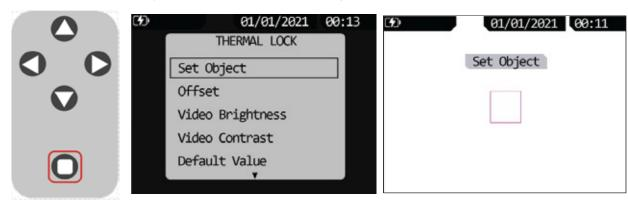
After capturing the object with Set Object, go to the Offset option. Enter the option by pressing the Enter button: an image will be displayed on the screen as shown. Point at a target with the scope and change the Offset value with the cursor until you find an image with the best detail.
