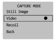
To capture an image or video, return to the Main screen, focus on a target and press the right arrow button. If you selected the Still Image Capture mode, the camera will take a picture. If you selected the Video Capture mode, the camera will start recording video. To stop video recording press the Enter button again.
