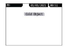
1) When the message cold object appears, close the lens cap, then press and release the Enter button. A message will appear saying Capturing. Wait until you see the message Cold Object Set and then press and release the Enter button to go to the next step.
