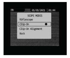
To change to Clip-On mode, scroll to Clip-On and press the Enter button. The image size will be reduced to 368x278 or 736x555 px.
